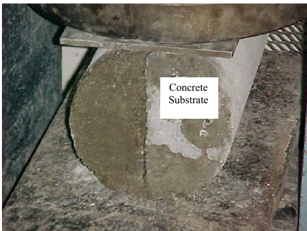
Fig. 2. Cylindrical splitting specimen at failure.
