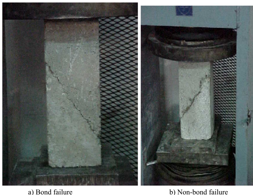
Fig. 5. Slant shear specimens after failure.
