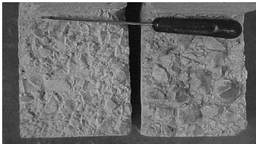
Fig. 4. Low (left) and high (right) roughness surface preparation.
