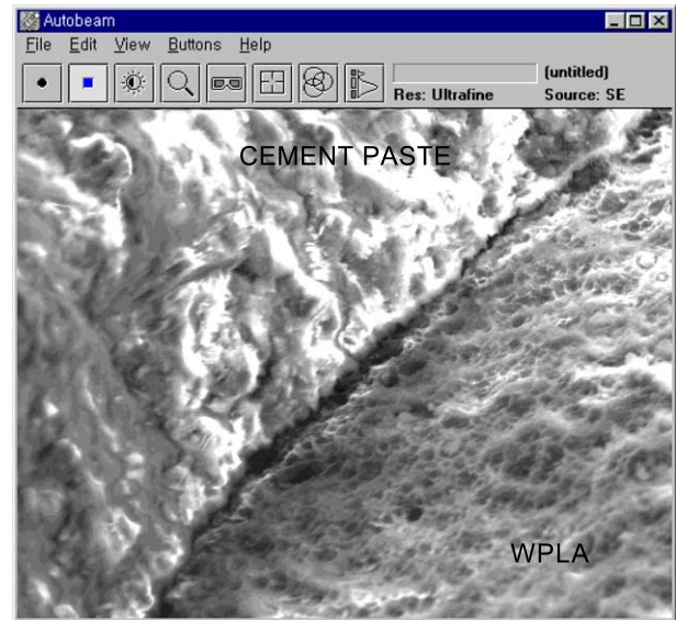
Fig. 7. Transition zone between cement paste and WPLA in mortar (28 days, magnified \times 700 ).
