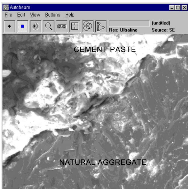
Fig. 6. Transition zone between cement paste and natural aggregate in mortar (28 days, magnified \times 700 ).
