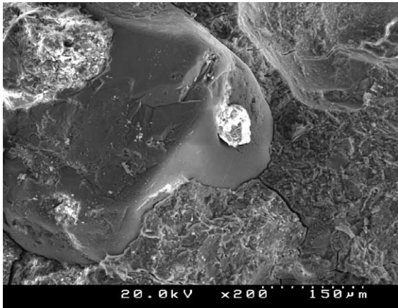
Fig. 7. Cracks in the paste and at the paste–aggregate interface in concrete C1.
