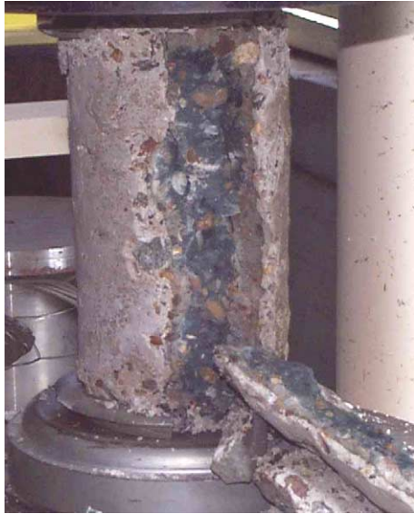
Fig. 4. A crushed cylinder of C5 after 168 days immersion in 1% sulphuric acid.
