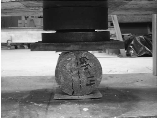
Fig. 1. Test setup for splitting tensile strength.
