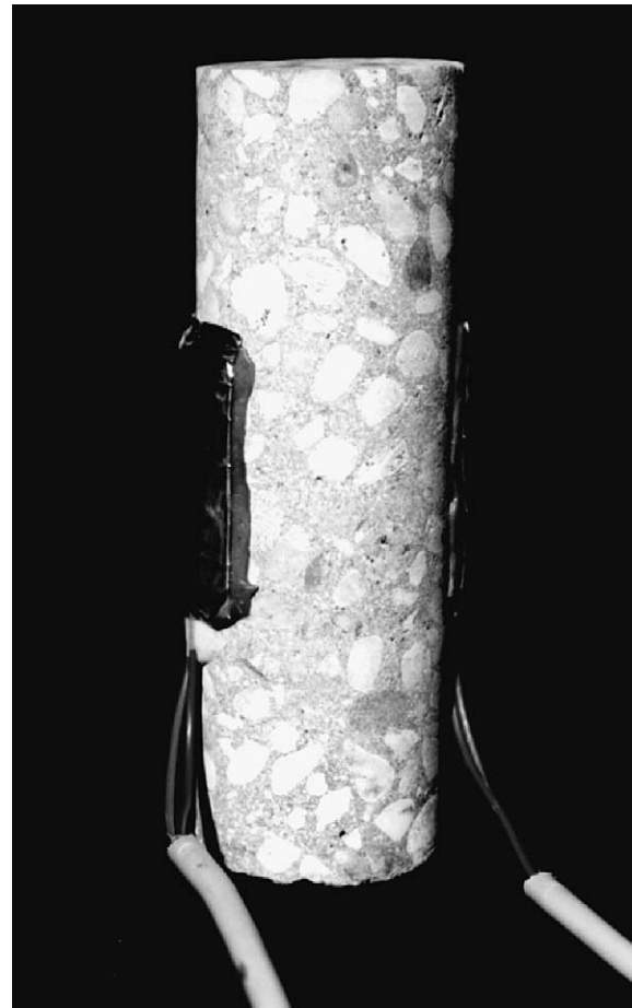
Fig. 2. Arrangement of the thermoresistors on the test piece.
