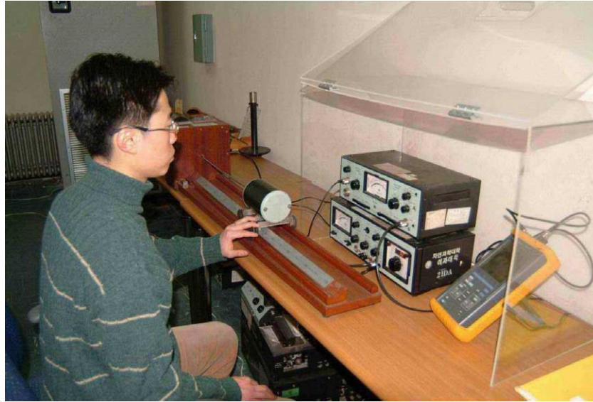
Fig. 1. Measurement of absorption coefficient by impedance tubes.
