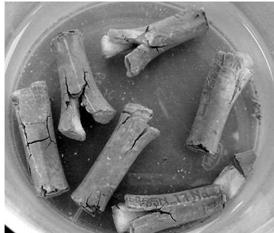
Fig. 15. Type I cement paste samples with w/c of 0.485 showed multiple cracks and some spalling at 108 weeks of exposure.
