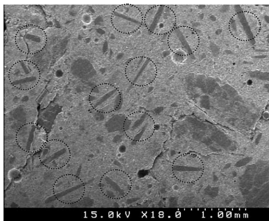
Fig. 4. Uniform distribution of E-glass in concrete.
