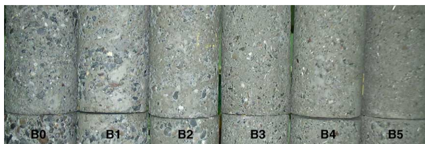
Fig. 15. Surface defect of concretes after five-cycle exposure for mix B.
