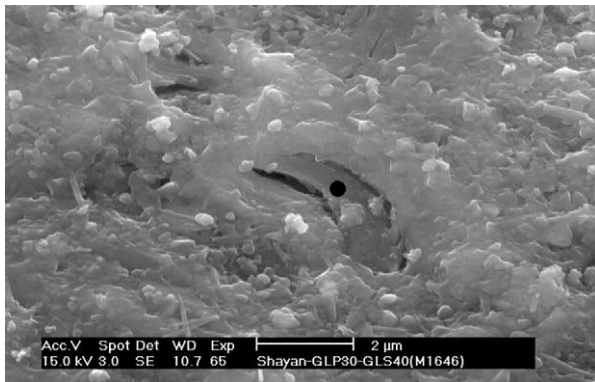
Fig. 18. SEM view and EDX composition of the relics of a very fine glass particle in Mix 7, reacted with cement to form a CSH-like material. Note high Na and K contents.
