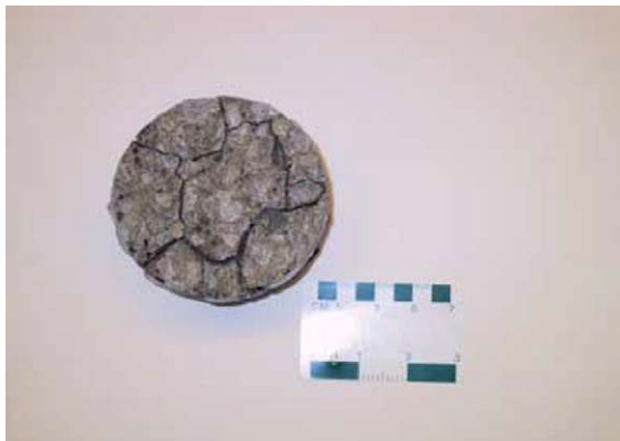
Fig. 1. Severely cracked core of 0.45 w/c Portland cement concrete heat cured at 95 °C, stored outdoors for 28 days and ponded in 2.8 M NaCl for 90 days. It was removed from NaCl and kept in –18 °C freezer when it cracked after about 6 months of storage.
