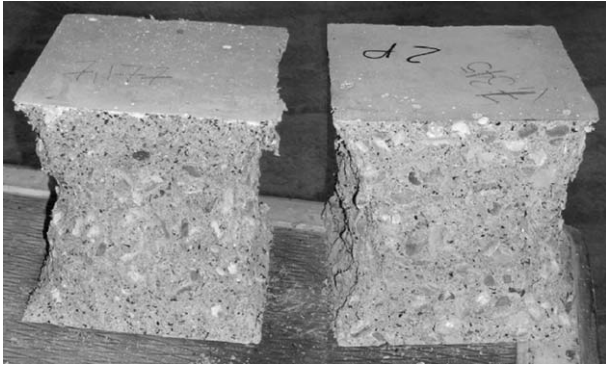
Fig. 1. SCRC cubes after rupture.
