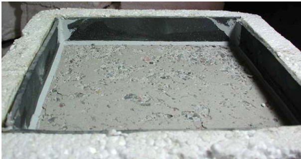
Fig. 4. Surface scaling of 550 g/m 2 of a slab test specimen after 56 freeze–thaw cycles.
