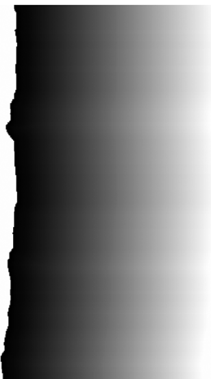
d) EDM of paste from the aggregate boundary. The grey value of each pixel in the paste increases with its nearest distance from the boundary.
