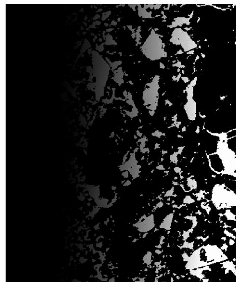
e) Distance map of the pore phase from the aggregate boundary. The brightness of each pore pixel represents its nearest distance to the aggregate.
