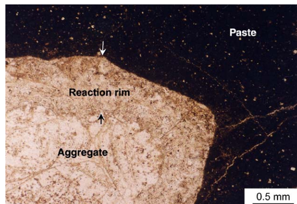
Fig. 6. Petrographic micrograph of ZP-K-1.8 KOH autoclaved for 150h, polarized light.
