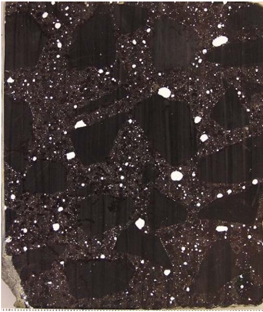
Fig. 2. Appearance of sample #2 after being coloured black and white BaSO 4 powder filled into the air voids.
