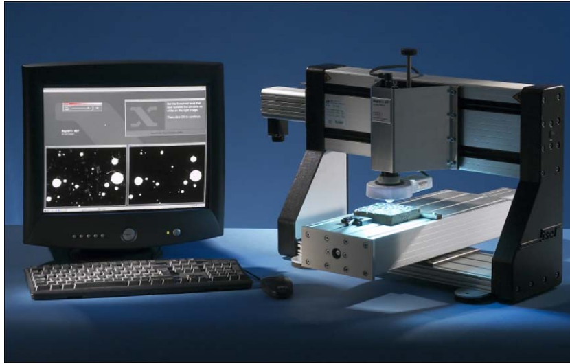
Fig. 5. The RapidAir system for automatic analysis of the air void system in hardened concrete.
