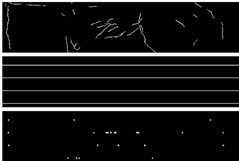
Fig. 5. Estimation of crack pattern orientation by means of the oriented secants method—logical binary operations between two images.
