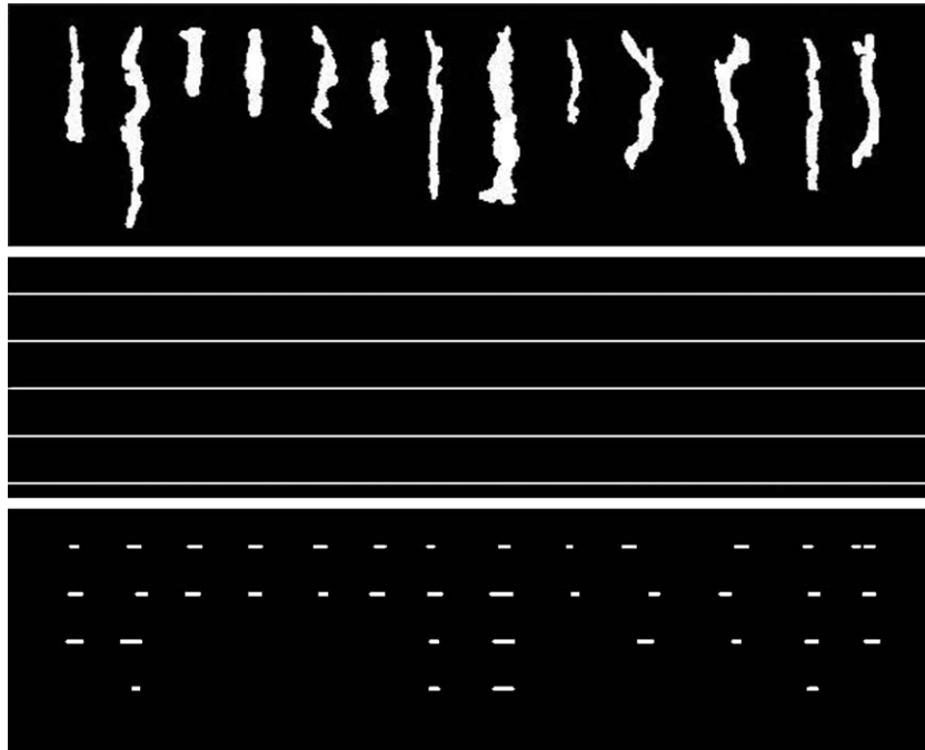
Fig. 6. Logical operation of crack image and image of parallel lines.
