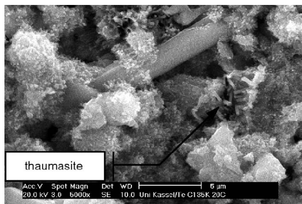
Fig. 11. SEM pictures of mortar sample C135K stored at 20/65.
