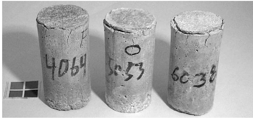
Fig. 1. From left to right: 0.40, 0.50, and 0.60 w/c mortar cylinders after 84 days in cold MgCl_2 brine. Cylinder dimensions are 50 mm in diameter and 100 mm in height.
