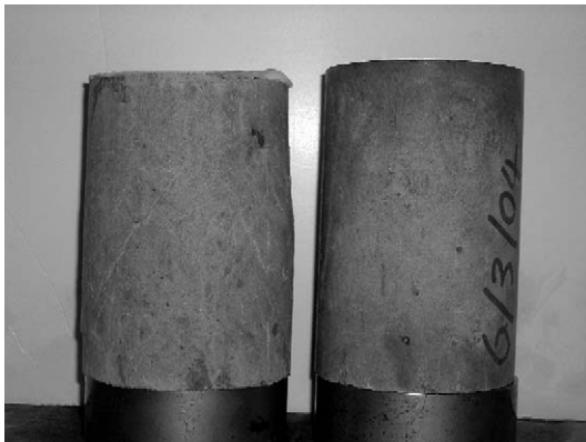
Fig. 5. Triaxial compression of 100×150 mm cylinder under lubricated loading platen. (Left: after test, Right: before test).
