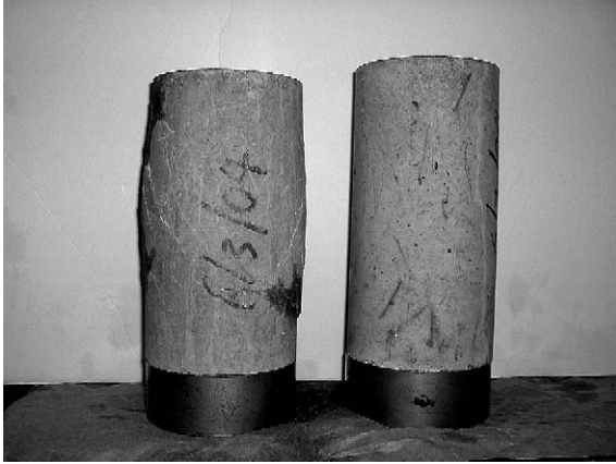
Fig. 4. Triaxial compression of 100×200 mm cylinder under rigid loading platen. (Left: after test, Right: before test).
