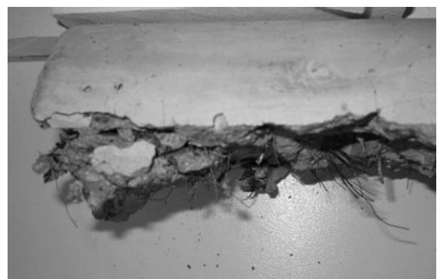
Fig. 5. Splitting tension failure interface (6% steel bead content).
