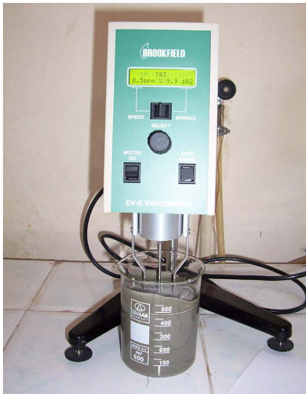
Fig. 3. Brookfield DV-E type viscosimeter.
