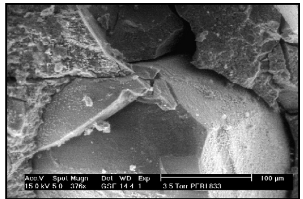
Fig. 17. ESEM image of lime sand pellet with raw perlite (C/S=0.83).
