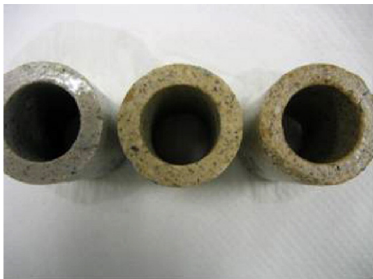
Fig. 1. Photography of tube sample — intact sample is on the left and others are degraded.
