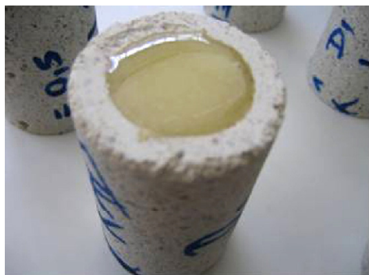
Fig. 7. Specific tube preparation for gas permeability measurements.
