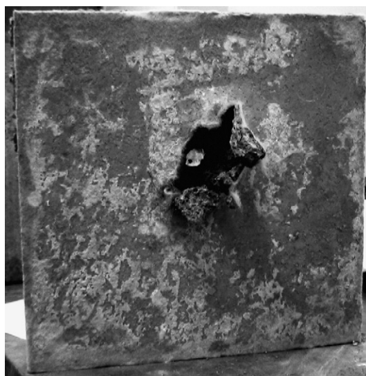
Fig. 5. Damage of back face with bonded fabric in a 3.81-cm-thick sample protected by Polypropylene fabric (PP3 ® ).
