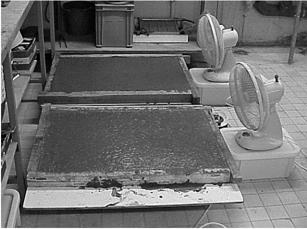
Fig. 3. Double restrained slab cracking test. (Air flow velocity set to 3 m/s).
