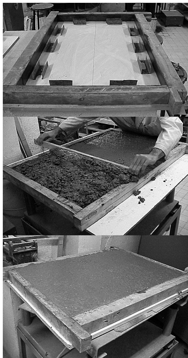
Fig. 2. Standard concrete specimen preparation for the double restrained slab cracking test (Kraai modified test).
