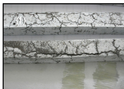
Fig. 2. Expansion curves with the time (a) OPC1 and FA1 mortars (100% of SA) (b) OPC2 mortars (100% of RA); FA2 mortars (No data) (c) OPC3 y FA3 mortars (“pessimum” proportion aggregate). Image of the mortars (d) OPC1 (100% of SA) on the 90th day (e) FA1 (100% of SA) on the 90th day (f) OPC2 (100% of RA) on the 56th day. The features of all mortars are shown in Table 3.
