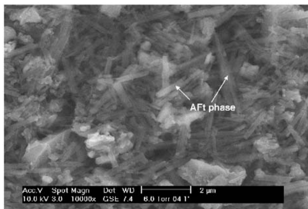
Fig. 15. ESEM micrograph of AC_{anhd} after 1 min of hydration (unit length 2 \mu m ).
