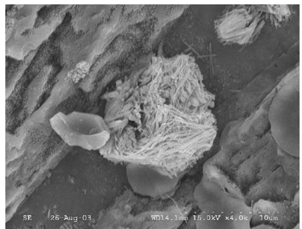
Fig. 4. Ettringite spherulite in Cement 3 cross-section.
