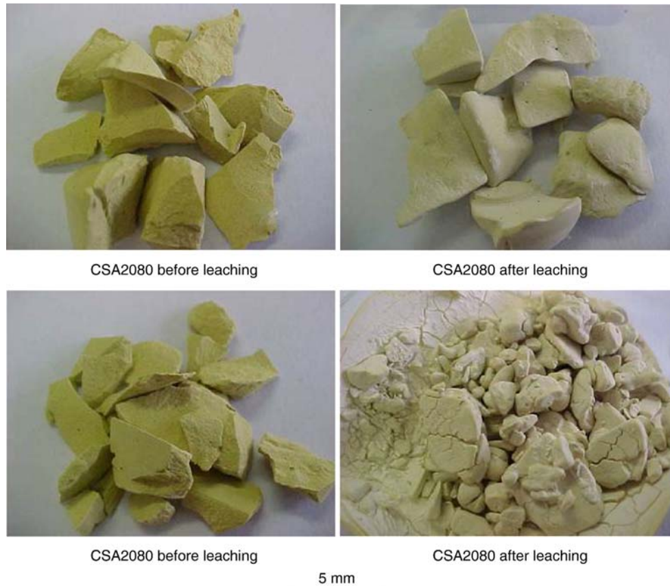
Fig. 2. Behaviour of pastes containing sodium chromate during leaching at 28 days.
