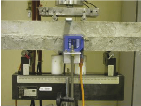
Fig. 1. Experimental set-up for four-point bending fatigue tests.
