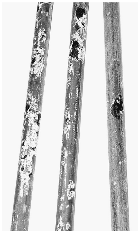
Fig. 8. Photo of steel bars after breaking specimens at the end of corrosion testing period. From left: 1) ORG1a 2) Control 3) ORG2a.
