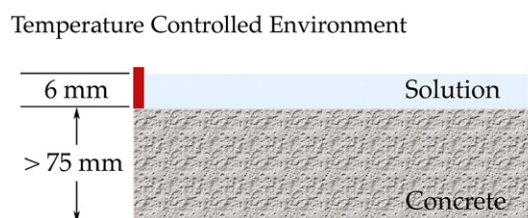
Fig. 2. Schematic of the ASTM standard C672 test method.
