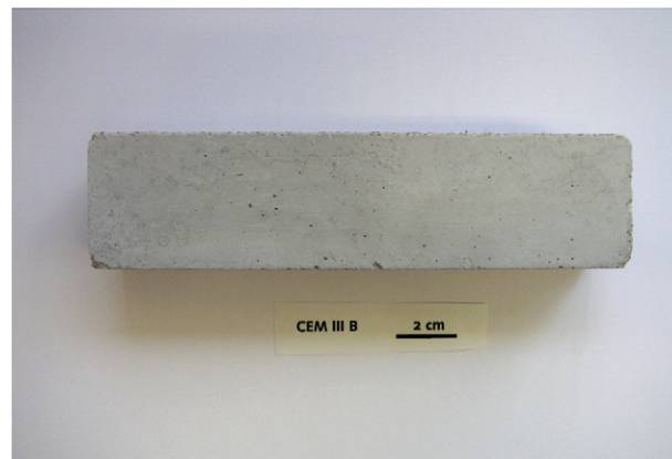
Fig. 5. Mortar bar made from blast furnace slag cement after 4.5 years of exposure ( \text{SO}_4^{2-} = 1500 mg/l and 8 °C).
