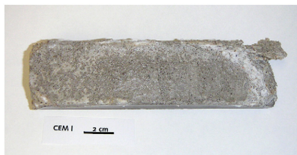
Fig. 2. Mortar bar made from Portland cement after 3 years of exposure (SO 4 2− = 1500 mg/l and 8 °C).
