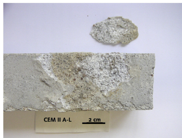
Fig. 3. Mortar bar made from Portland limestone cement under addition of 5% silica fume after 3 years of exposure (SO 4 2− = 1500 mg/l and 8 °C).
