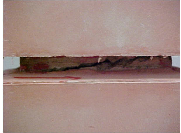
Fig. 12. Shear crack dilation (direct shear test at 3 MPa).
