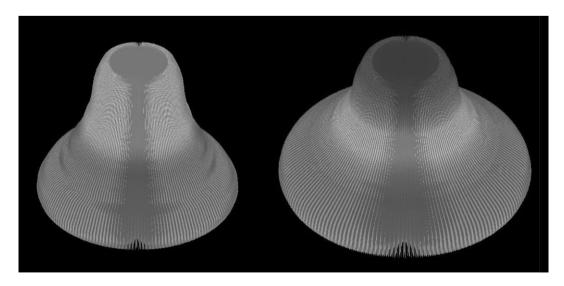
Fig. 2. Examples of obtained shapes for the ASTM Abrams cone (left) yield stress=2600 Pa (right) yield stress=2000 Pa. Density=2500 kg/m³ for both simulations.
