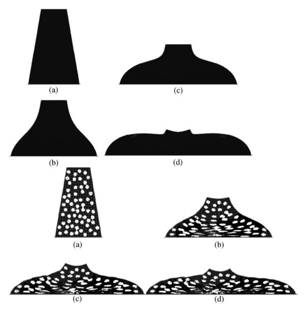
Fig. 9. (top) Numerical simulation of the slump flow test using a homogeneous approach (bottom) Numerical simulation of the slump flow test using a heterogeneous approach.
