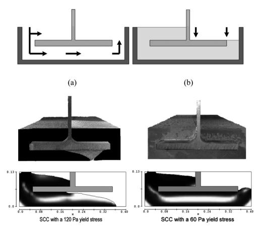
Fig. 4. Casting of a concrete pre-cambered composite beam. (upper part left) Schematic showing the first phase of the casting; (upper part right) Schematic showing the second phase of the casting; (lower part) Comparison between experiments and numerical simulations for two SCC with yield stresses equal to 120 Pa (left figures) and 60 Pa (left figures). Black shading emphasizes the casting defect on the upper left picture, Units are meters (from [10]).
