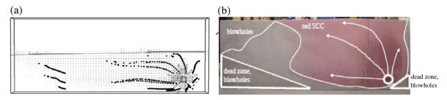
Fig. 3. a) Simulated velocity field and particle paths in the time interval from 120 to 250 s. b) Observed flow behavior in the experiment (dead zones, particle path of the red SCC, segregation, and surface quality). The injection point is located at the bottom right corner of the formwork (white circle).
