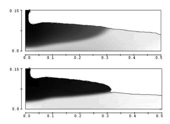
Fig. 6. Numerical simulations of the multi-layer casting phenomenon using the thixotropic model proposed by Roussel [11] with  $\tau_0$ =50 Pa,  $\mu_p$ =50 Pa.s,  $A_{thix}$ = 0.5 Pa/s,  $\alpha$ =0.005. (upper figure) For a 5 min resting time, the two layers mix perfectly; (lower figure) for a 20 min resting time, the two layers do not mix at all (units are meters).
