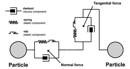
Fig. 7. A standard contact law between two particles in DEM. According to the separating distance and relative velocity of the particles, normal and tangential interaction forces between particles can be calculated.
