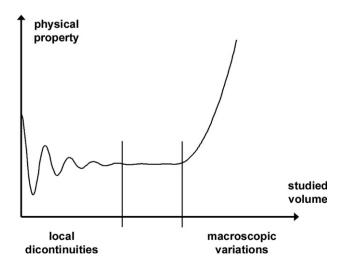
Fig. 1. Variation of a physical property averaged over a given volume of material as a function of the volume size.
