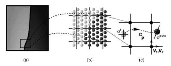
Fig. 8. Schematic representation of FEMLIP (a) Interfaces are set by applying different behavior to material in space (b) A set of Lagrangian particles are used as integration points and to track material properties (c) Particles are moved according to nodal velocities and history dependant variables are stored on particles.
