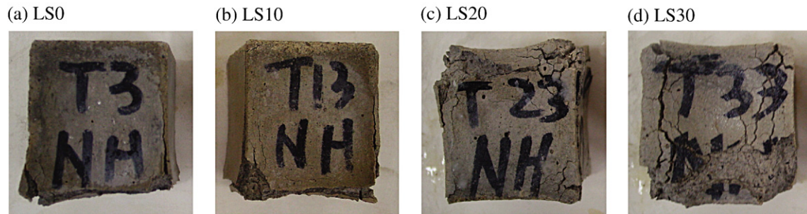
Fig. 7. Cube mortar specimens exposed to sodium sulfate solution (360 days).
