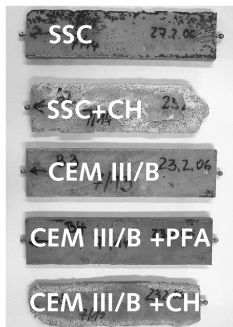
Fig. 1. Mortar bars after 12 months of exposure to Na 2 SO 4 solution (SO 4 2− = 3000 mg/l) at 8 °C.
