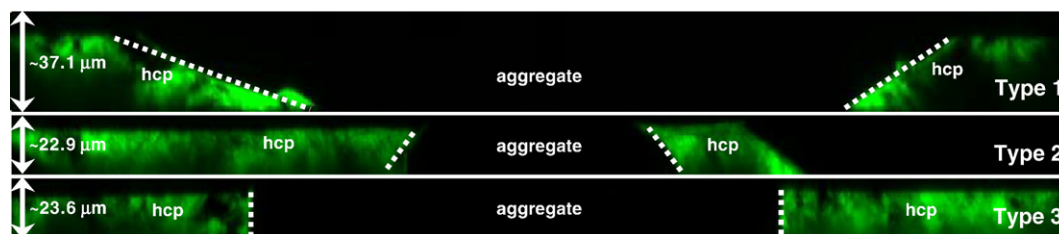
Fig. 3. Example of sub-surface aggregate interfacial geometries (XZ profiles through confocal image stacks). Note: Imaging depth shows depth of confocal data set, not thickness of thin-section.
