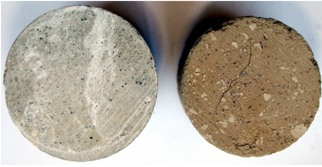
Fig. 4. Surface difference between sound and chemically degraded cement paste samples.
