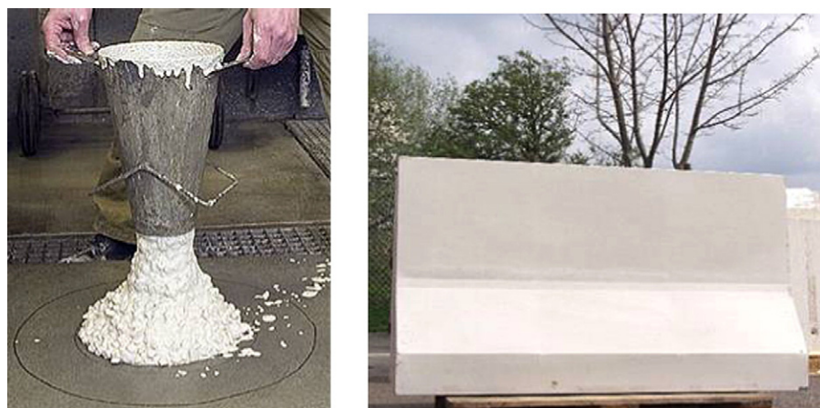
Fig. 2. Left: White SCC slump flow test. Right: White SCC provides flawless surfaces.
