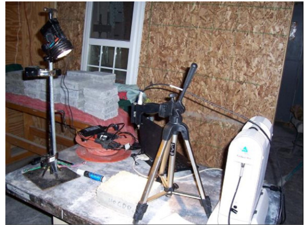
Fig. 1. Experimental set-up for collecting the surface spectral reflectance of concrete blocks.
