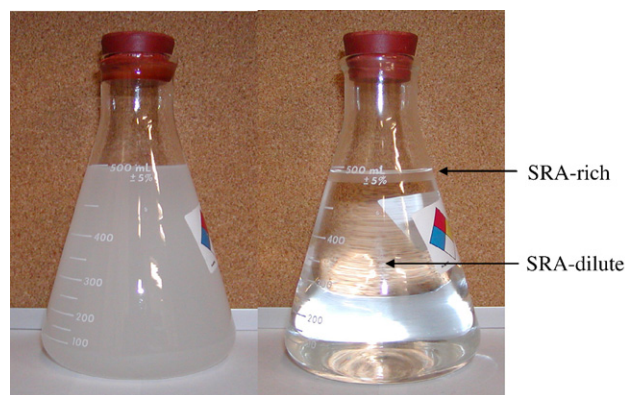
Fig. 3. Separation of emulsion made by mixing 10% SRA in the synthetic pore solution; (left) immediately after mixing, (right) kept at rest for 12 h.
