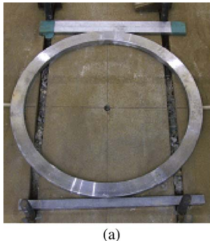
Fig. 5. (a) The annular steel support, (b) the biaxial flexure test and the initial crack development, and (c) the uniaxial modulus of rupture test for the reference test result.
