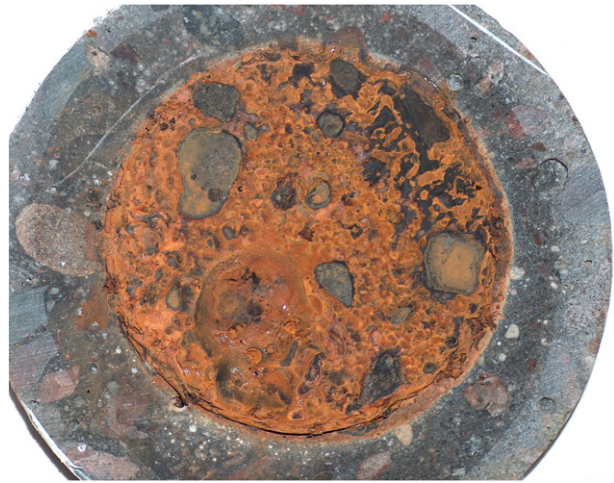
Fig. 6. Deposits formed on the anodic side of the concrete sample. The deposition of these materials occurs mainly on the cement paste zones, and not over the aggregates.
