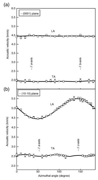
**Fig. 3.** Spatial dispersion of the quasi-longitudinal and quasi-transverse acoustic velocity in the two crystallographic planes of ettringite. (a) basal plane  $(-0.1 \ 0.14 - 0.04 \ 1.91)$ . (b) Plane (1 - 0.15 - 0.85 - 0.57). LA: quasi-longitudinal acoustic velocity. TA: quasi-transverse acoustic velocity. Circles: measured velocities. Lines: velocities calculated according to the elastic constants determined in this study ( Table 2).
