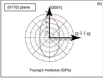
Fig. 5. Polar plot of the Young's modulus along directions in two orthogonal crystallographic planes of ettringite. (a) (0001) plane. (b) (01 - 10) plane.
