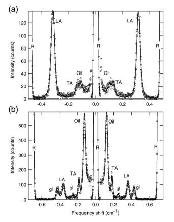
**Fig. 2.** Brillouin spectra collected from the two sample platelets. (a) basal plane (-0.10.14-0.041.91). (b) plane (1-0.15-0.85-0.57). LA: sample quasi-longitudinal acoustic mode. TA: sample quasi-transverse acoustic mode. R: elastically scattered light. Oil: mineral oil. gl: glass.
