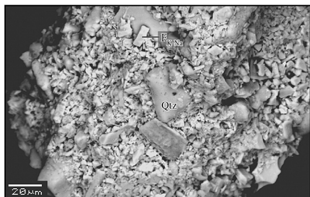
Fig. 3. Scanning electron micrograph of a grain from the poz-1 sample. Voltage is 20 kV. The scale bar indicates a length of 20 µm.
