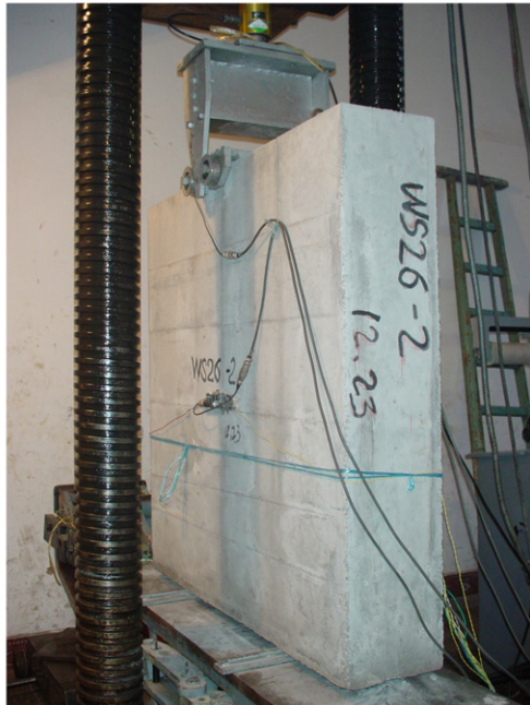
Fig. 3. Real test set-ups. (a) Three-point bend beam test. (b) Wedge splitting test.
