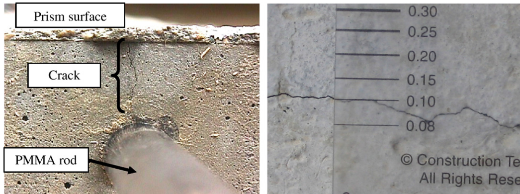
Fig. 4. 0.1 mm longitudinal crack, caused by thermal expansion coefficient difference between PMMA and concrete.
