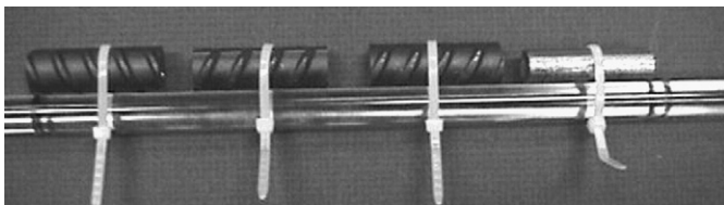
Fig. 1. Corrosion probes showing three black steel elements and one stainless steel element.
