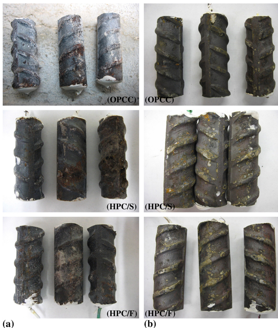
Fig. 11. Top steel probes recovered from three of the prisms with longitudinal crack after 128 weeks of exposure to de-icing salt: (a) before removing the corrosion products, (b) after removing the corrosion products.
