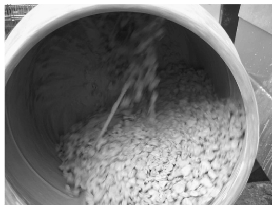
Fig. 4. WSA milling process using silica pebbles as grinding media in a drum and pebble mixer.
