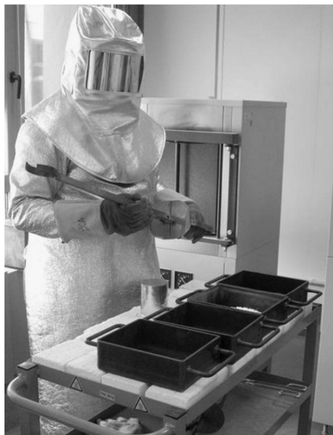
Fig. 6. Sample during quenching — the sintered material has just been poured from a platinum crucible into a big steel receptacle to enhance cooling.
