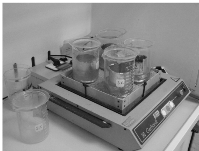
Fig. 5. Crucible cleaning setup with HCl in a heated sand bed. Petri dishes covering the glass beakers reduce the evaporation rate of the acid, but the apparatus still needs to be placed under a fume hood.
